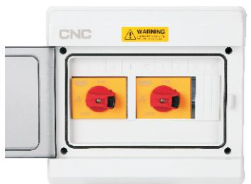
Isolation boxes are most commonly used in two way / three way / four way / six way solar home roof systems. The UV-resistant and fire-resistant PC case protects the DC components from sunlight and water ingress, and the box lid is lockable. Included in the box are two din rail mounted DC switches, up to 40A per IEC 60947.3 and AS60947.3 PV2, with lockable handles for safe use and maintenance.
